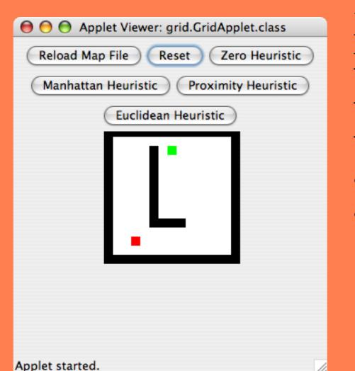
In this project, students implement the A\* shortestpath algorithm, with a variety of admissible heuristics to shape the search process. By dropping it into a GUI, they can visualise the real effects of different choices in the search policy. To the left is a screenshot of the GUI and an initial map; below are that map's exploration according to four different heuristics.
